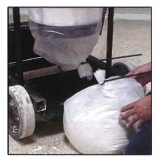
Cut between the ties and dispose of the filled bag.
