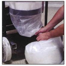
Continuous plastic tube is pulled downward and divided into single bags of any size.
